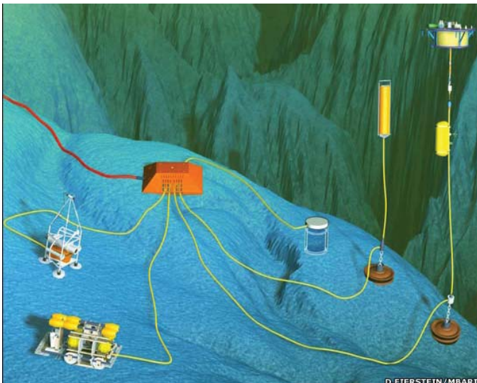
The main Mars science node sits at a depth of almost 900m. Running off the node will be a series of instruments that constantly return data to shore.
